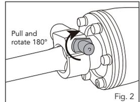
2. Insert the shank of the accessory into the nose of the tool. Ensure the notch in the shank is positioned as per the illustration shown. The notch in the shank of the accessory has to face the flat of the accessory holder as illustrated. If the notch is in an incorrect position, the shank will not lock into position.
