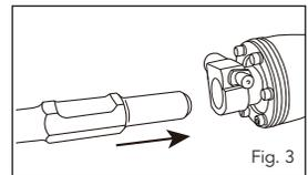
3. Lock the shank into the nose of the tool by pulling out the quick release bit lock (8) and rotating it 180°.
